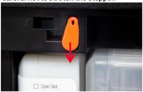
With the stopper in place the printer will read the door as closed.
